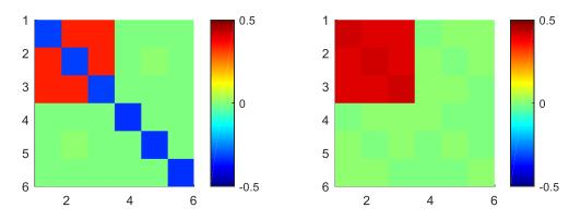
Figure 2. The two unresolved linear combinations of elastic parameters for a "both X and V" inversion, here shown as  $6 \times 6$  Voigt matrices  $C_{ij}$ . They correspond to two different linear combinations of the Lame parameters  $\lambda$  and  $\mu$ . Only the elements  $C_{14}$ ,  $C_{15}$ ,  $C_{16}$ ,  $C_{24}$ ,  $C_{25}$ ,  $C_{26}$ ,  $C_{34}$ ,  $C_{35}$ ,  $C_{36}$ ,  $C_{45}$ ,  $C_{46}$  and  $C_{56}$  are fully-resolved.
