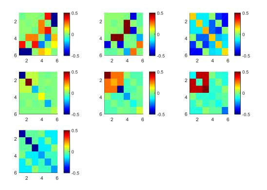
Figure 3. The seven unresolved linear combinations of elastic parameters for a V-only inversion, here shown as  $6 \times 6$  Voigt matrices  $C_{ij}$ . Only the elements  $C_{14}$ ,  $C_{25}$  and  $C_{36}$  are fully-resolved.
