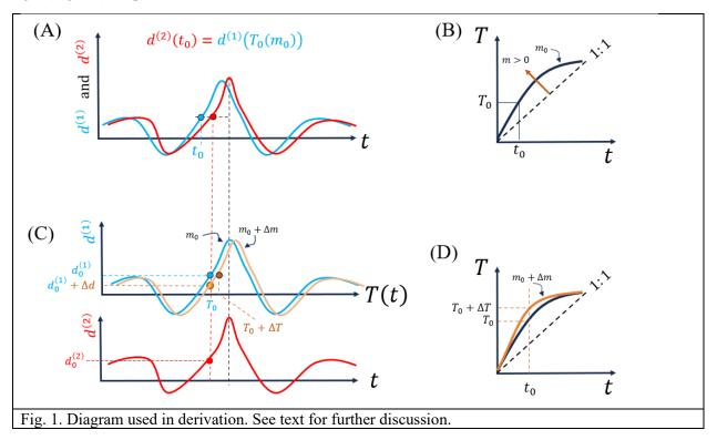
Now suppose that the choice  $m = m_0$  lines the times series up pretty well in the vicinity of a time  $t_0$ . A small perturbation  $\Delta m$  around  $m_0$  causes a small perturbation  $\Delta T$  in  $T_0 \equiv T(t_0, m_0)$  (Fig. 1B).
