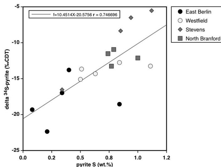
**Figure 12.** Pyrite sulfur isotopic compositions vs. pyrite sulfur concentrations in the Westfield member of the East Berlin Formation. Average sulfur isotopic compositions from the deeper sites (North Branford =  $-12.0\text{‰}$ ,  $n=4$ ; Stevens =  $-9.2\text{‰}$ ,  $n=4$ ) are more positive than shallower sites (Westfield =  $-13.8\text{‰}$ ,  $n=5$ ; East Berlin =  $-18.2\text{‰}$ ,  $n=5$ ) (Data from Leonard, 2013).
