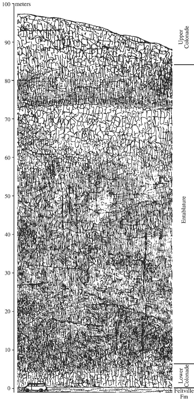
Figure 23. Composite drawing of the type section of the Preakness Basalt along Interstate Route 280 about 2.25 km west of the type section of the Orange Mountain basalt (Figure 22). Traced from a composite of a continuous series of photographs with the dip removed and compiled vertically (Olsen, 1980b).
