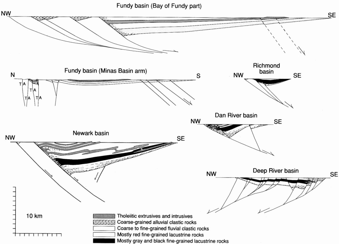
**Figure 2.** Cross sections of selected Newark Supergroup basins (see Figure 1 for locations). Note half-graben shape of all basins except the Minas basin arm of the Fundy basin, which lies along the largely strike-slip part of the basin where it trends east-west. Cross
