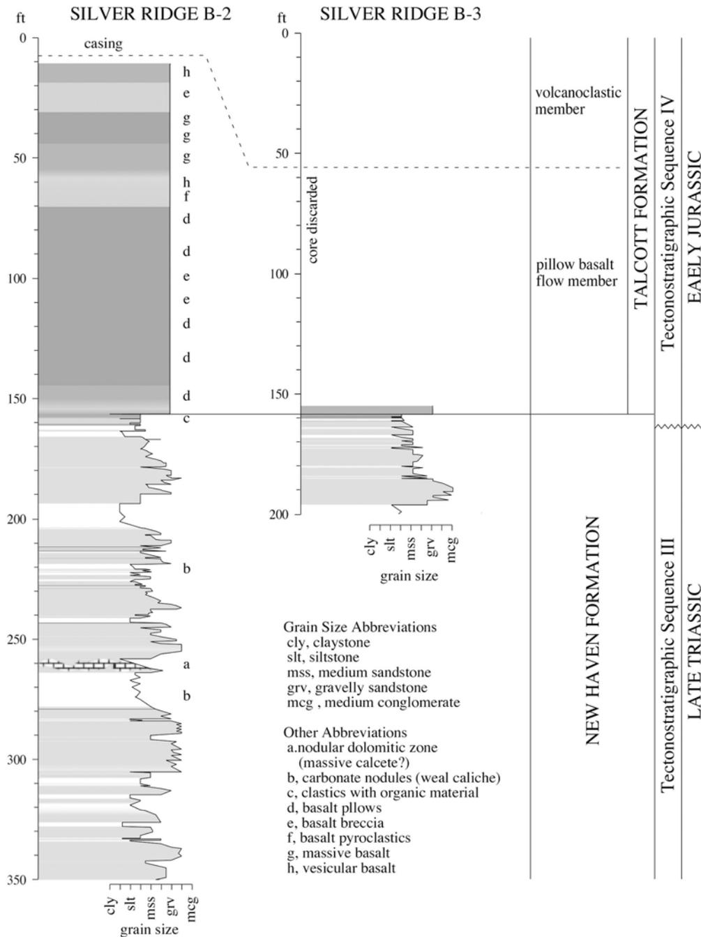
Figure 19. Cores B-2 and B-3 from Silver Ridge (Stop 6) on display at Stop 5b.
