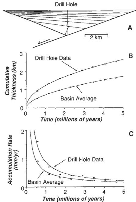
FIG. 4.—Half-graben filling model. (A) Cross section of half-graben loosely based on the geometry of the Atlantis basin (fig. 1), in which stratal surfaces, corresponding to time slices of 550,000 yrs, delineate areas of  $1.5 \times 10^6$  m<sup>2</sup> which were iteratively fit to the basin. Cumulative sediment thickness (B) and accumulation rate (C) show similar trends as in a full-graben (cf. fig. 9).
