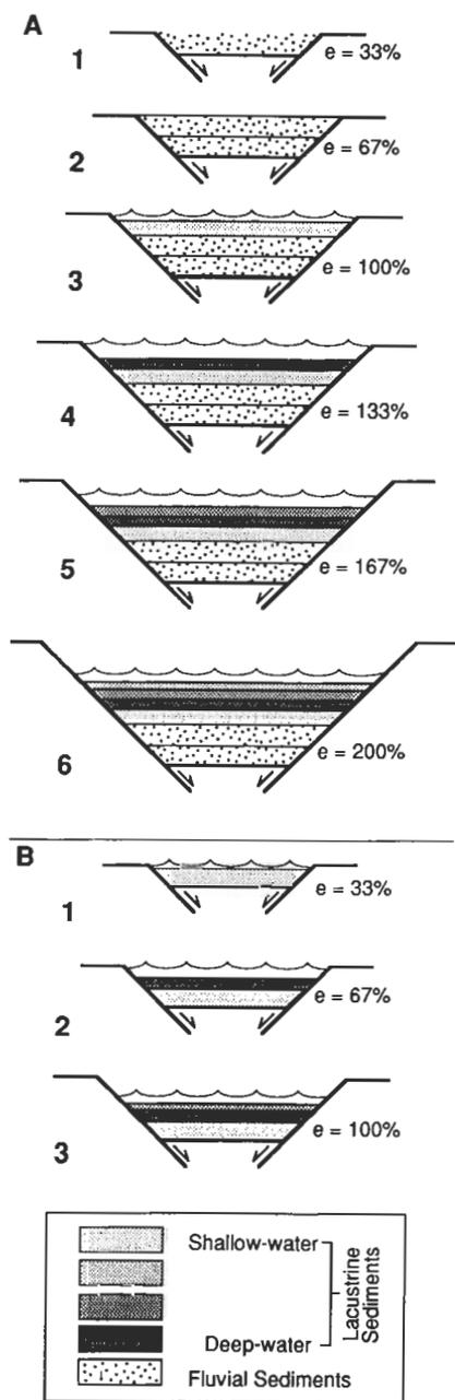
FIG. 3.—Diagrammatic representation of the salient features of the filling of a full-graben under conditions of uniform subsidence and constant volume input of sediment per unit time; *e* equals percent extension. See text for further explanation.
