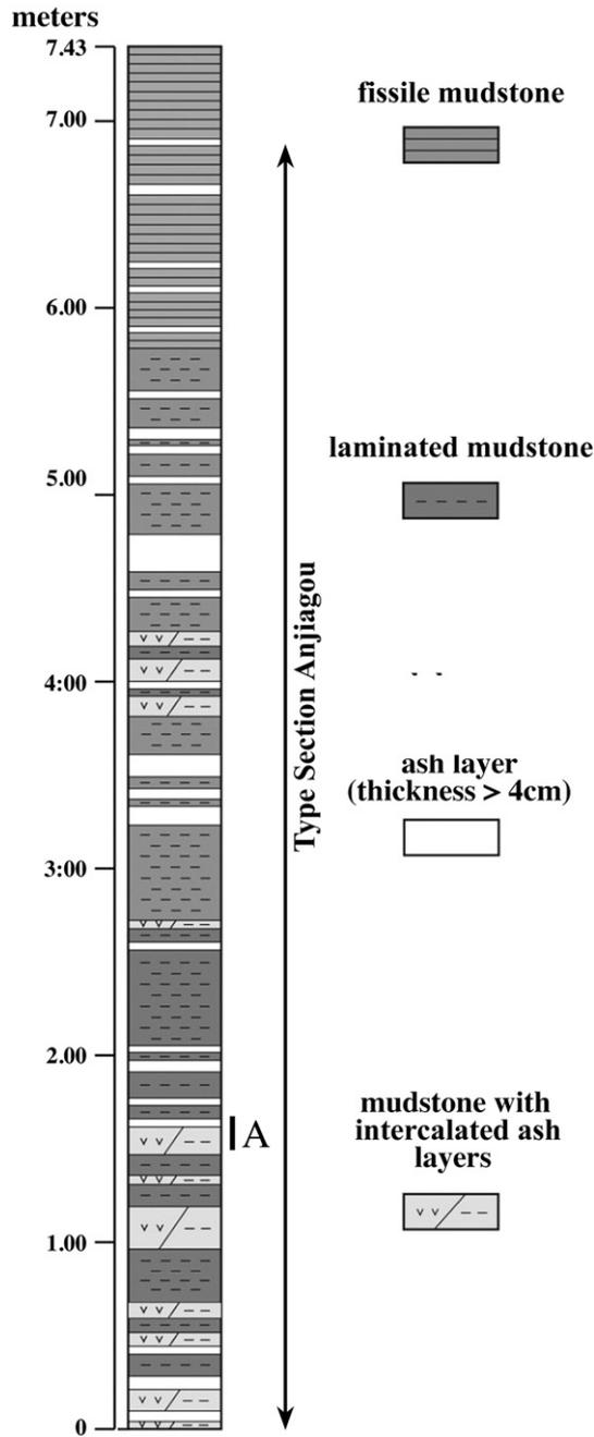
Fig. 17. Type section Anjiagou Bed, Sihetun Museum modified from Zhang and Sha (2012). A indicates position of samples shown in Fig. 18.
