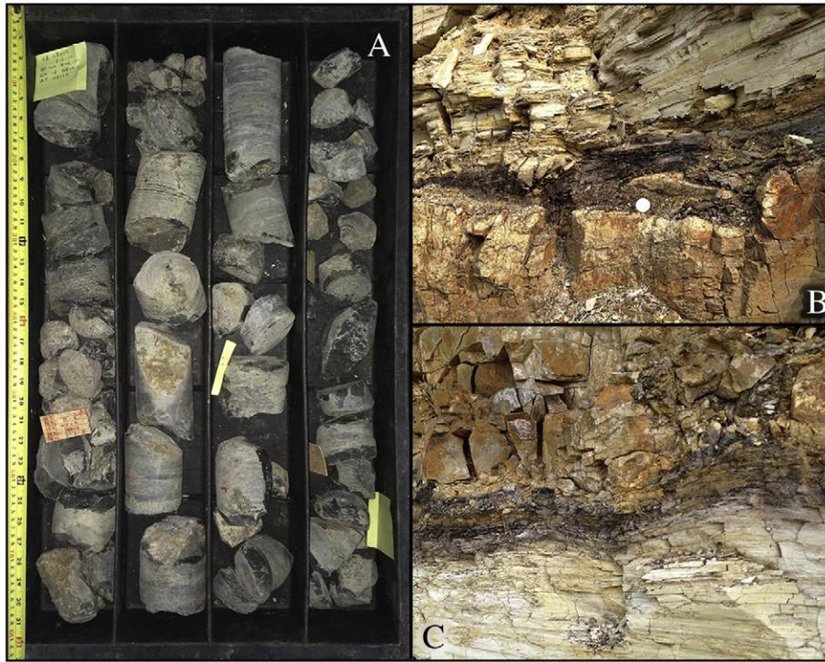
**Fig. 16.** Intrusive igneous rocks: A, box 27 of Sihetun no. 1 core (0.0–4.1 m ACD; 0.0–5.5 SD); B: upper contact of igneous intrusion at exposure opposite and to the south of the Sihetun Landscape Fossil Bird National Geopark museum (41.588526°, 120.792492°), note black metamorphosed zone at contact – coin is ~2.5 cm; C, lower contact of intrusion at same location, the same scale as B applies.
