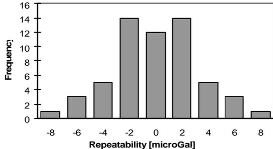
Figure 3: Distribution of gravity repeatability errors in the 2002 survey, based on 38 repeat measurements at 20 stations (deviations from station means).
