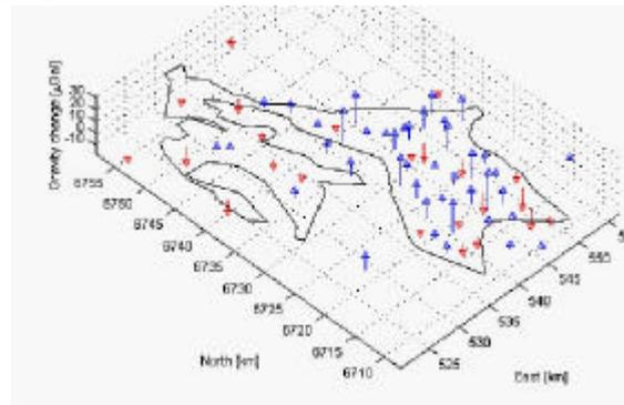
Figure 4: Time-lapse gravity changes 2002 – 2000. In this perspective plot, the rim of the hydrocarbon reservoir is drawn. Blue arrows are gravity increases, red are decreases, and a station is located at the tail of each arrow.
