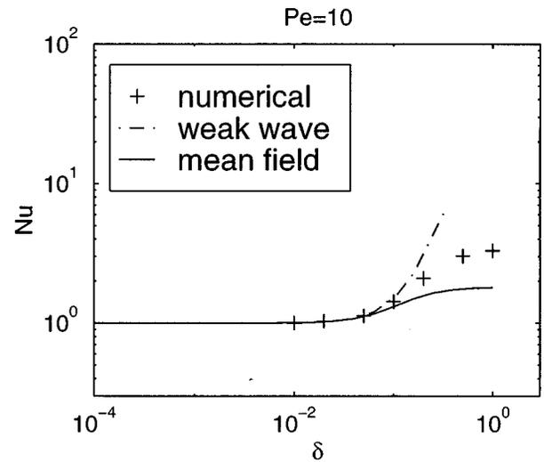
FIG. 1. Nu vs  $\delta$ , for  $\text{Pe} = 10$ . Full numerical solutions are shown for larger values of  $\delta$ , while the weak-wave asymptotic analytical solution is shown for the smaller values of  $\delta$ . Mean-field results are shown throughout the entire range.
