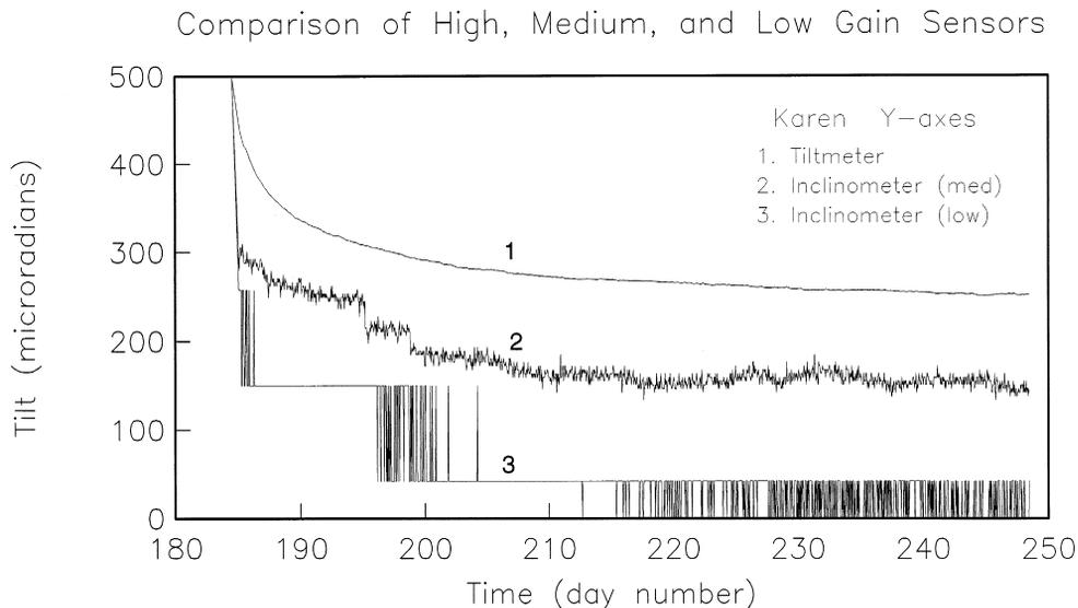
Fig. 6. Initial equilibration of Karen's Y channels, showing agreement between the high gain tiltmeters, medium gain inclinometers on the seismometer platform, and the low gain inclinometer on the equatorial ring.
