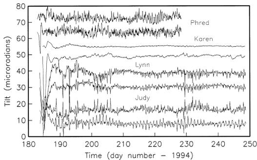
Fig. 8. Data from both *X* and *Y* channels of the bubble tiltmeters on four of the TILT-OBS with spline fit drift removed (Constable and Parker, 1988) to facilitate comparisons of short-term tilt rates. Energy that is coherent between instruments at tidal frequencies is evident. This is considered to be caused by tidal currents moving the instrument package; Karen was deployed inside the caldera and was thus sheltered from currents.
