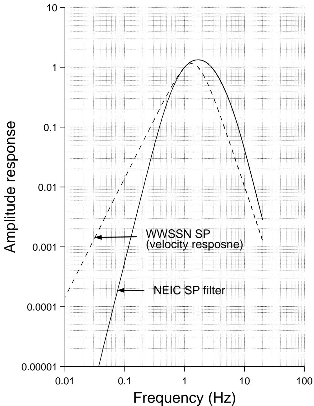
Figure 2: Comparison of the filter used at NEIC for  $m_b$  measurement and WWSSN short-period **velocity** amplitude response.
