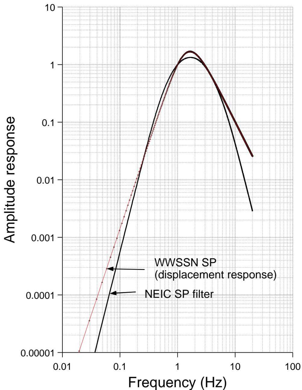
Figure 1: Comparison between the filter used at NEIC for  $m_b$  measurement and WWSSN short-period **displacement** amplitude response. NEIC SP response is actually two Butterworth, second order bandpass filters.
