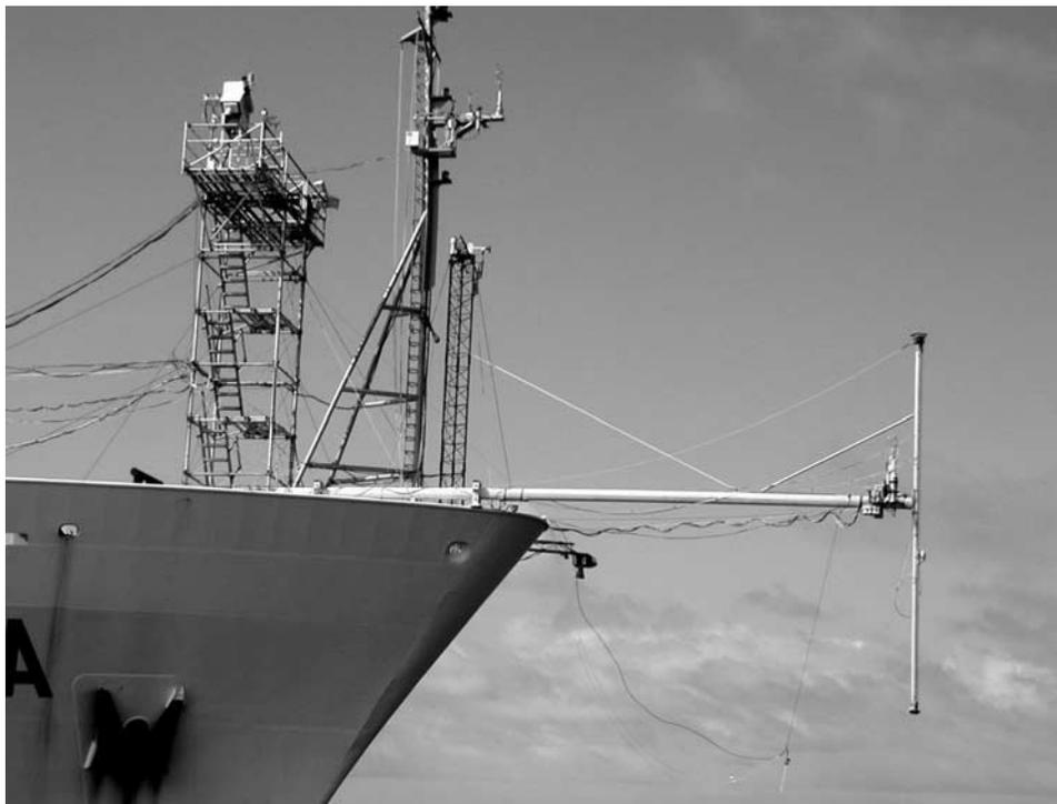
**Figure 3.** The experiment setup used during the GasEx experiment aboard the R/V *Ronald Brown*. The mast extended 10 m forward of the bow at its closest point. The figure also shows the flux package deployed by National Oceanic and Atmospheric Administration Environmental Technology Laboratory on the forward jackstaff and the infrared imagery system deployed by University of Washington Applied Physics Laboratory on the scaffolding.
